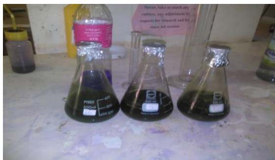
Fig. 2 : Powder Plants Samples Dissolved within Ethanol for Crude Extraction.
