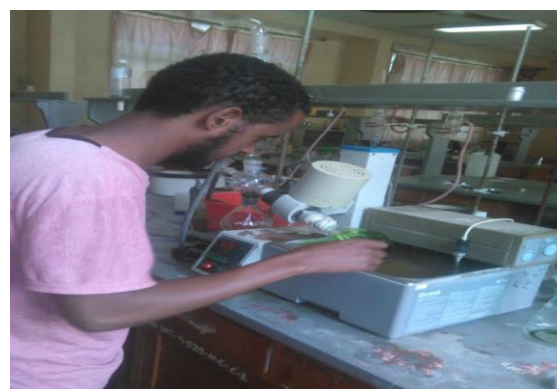
Fig.5 : Process of separation of crud extract from solvent using rotary evaporator
